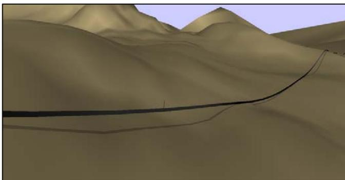
Figure 7: Free spanning pipeline on an uneven seabed
