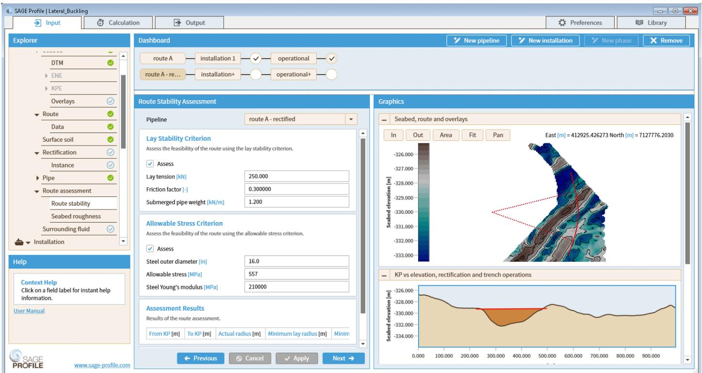
The Graphical User Interface streamlines the harvesting of input data to quickly set-up the model. In addition, it provides powerful visualization and reporting tools for interpreting output from the finite element engine.
