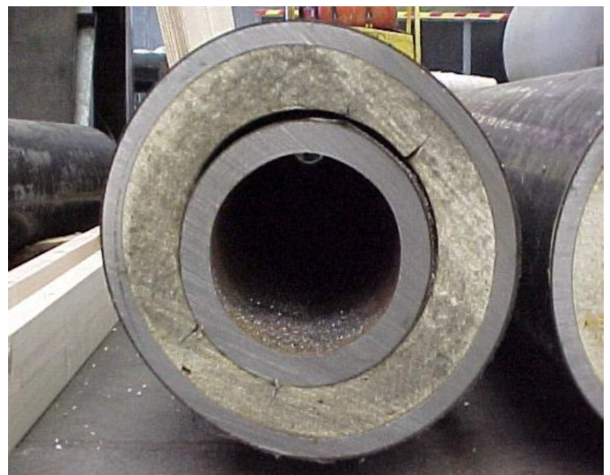
Figure 1: Cross section of a Pipe-in-Pipe system [1]
